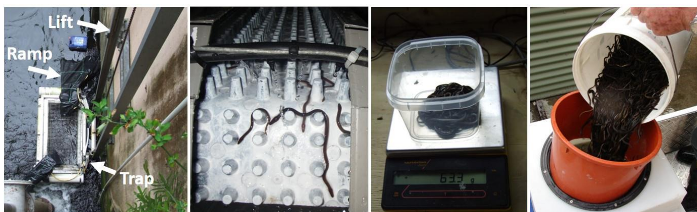
Figure 9: Elver trap-and-transfer activities. (Left to right) Elver trap at Karāpiro dam; An example of an elver ramp; Estimating the total elver catch using a sub-sample; and Transfer of elvers into transportation tanks for release. (Photos: Mike Martin and Jacques Boubée).
